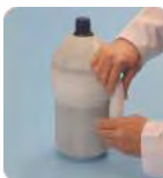
Step 6. When the bottle is empty, place the safe-handle on a flat surface to disengage. Hold the bottom handle with one hand. Using the other hand rotate the top in a counter clockwise direction until the lugs are disengaged. Remove the top from the bottom.
