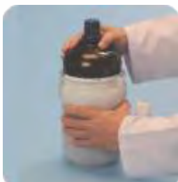
Step 2. Carefully place the bottle in the bottom portion of the Safe-Handle.
