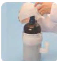
Step 3. Lower the Safe-Handle top over the neck of the bottle. Line up the indicator arrows to ensure assembly.
